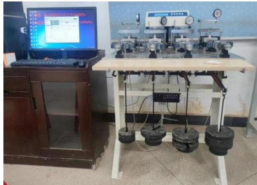
Fig.3: Type ZJ strain controlled four-linked direct shear apparatus
