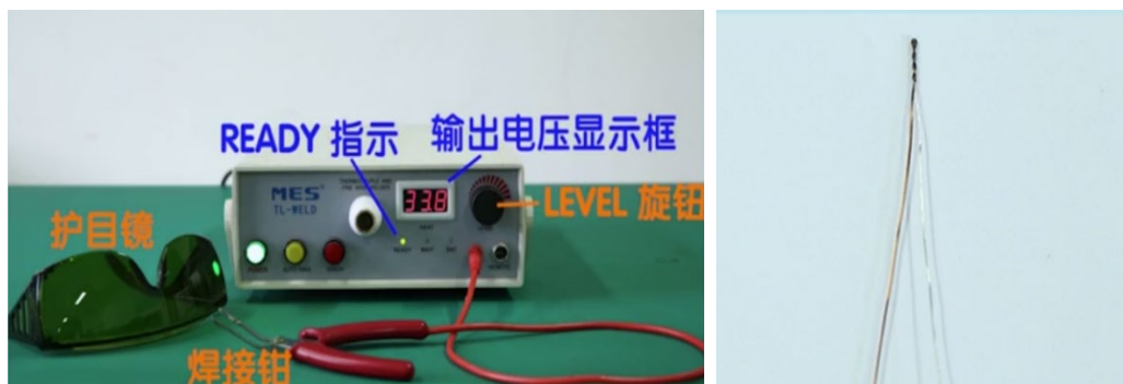
Figure 2. TL-WELD Type Thermocouple Welding Machine and Self-made Thermocouple
