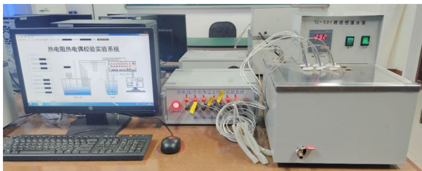
Figure 3. SY-3 Thermocouple Calibration System
